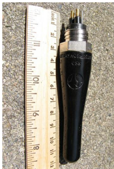
FIGURE 1.1 – Hydrophone Cetacean Research C55
