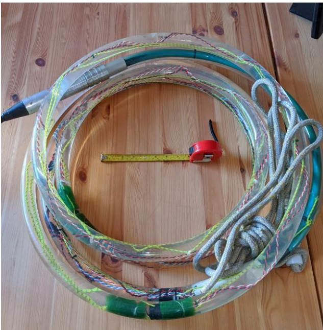
Figure 2. Example of one of the two identical hydrophone arrays used in the field. The two broadband elements in each array were separated by 3 m in an oil-filled tube to provide an optimal aperture for localising sperm whale clicks.
