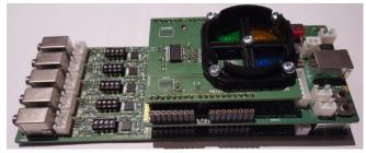
**Fig. 3**. The JASON sound card (SMIoT), 5 x 1 MHz sampling rate at 16 bits resolution, placed into the drone. The luxmeter was not used in this work.
